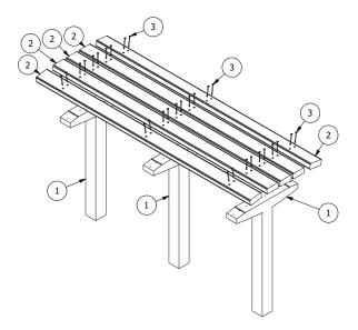
STEP 2: Auger Three 100mm holes at 700mm spacings approxmately 400mm deep. Place loose stone into bottom of the holes untill the required seat height is achieved. pour concrete into holes. Using a spirit level ensure seat is leveled correctly.
