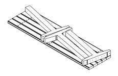
STEP 1: Place 95x45@1800 Profile on top of Eco T legs. Working from the outside in, screw through profile using 14gx75 screws. Be sure to align screws with marked holes in Eco Leg. Tourque screws down being careful not to over tighten.
