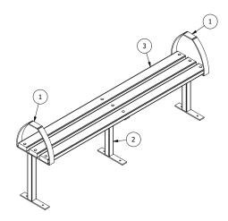
STEP 2: Place legs upright on level surface. Place three of the Dura Comp profiles on legs and lightly tap M8 bolts through profiles and holes through legs. Use washers and nuts then lightly tighten. Square completed seat then tighen all nuts being careful not to over tighten pulling bolts through profile.
