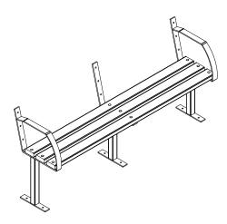
STEP 2: Place three of the Duracomp profiles on back rest and lightly tap M8 bolts through profiles and holes through legs. Use washers and nuts then lightly tighten. Square completed seat then tighen all nuts being careful not to over tighten pulling bolts through profile.
