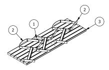
STEP 1: Place legs upright on level surface. Place three of the Duracomp profiles on legs and lightly tap M8 bolts through profiles and holes through legs. Use washers and nuts then lightly tighten.
