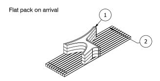
STEP 1: Place Legs (1) apart on ground. Screw bugle batten screws (3) through 50x50 profile (2) until the point shows through other side. Align with pre drilled holes in leg. Tighten screw down being carefull not to over tighten.
