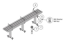
Place batten on legs. Lightly tap bolts through battens with hammer then secure using M6 nuts and M6 washers.
