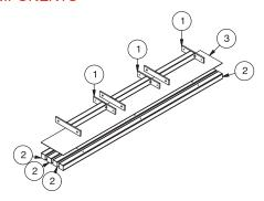
STEP 2: ATTACHING SEAT BATTENS
