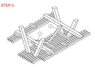
Fit braces. Position them from the centre of the table using the small cut back on braces towards the table top section. Back to back they will angle to main support. Use 10G x 75 screws to screw into place being careful not to push legs apart in the process.
