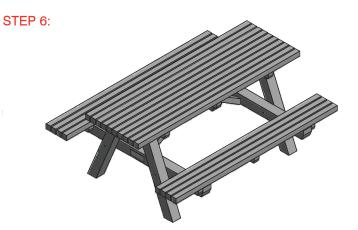
Being careful not to damage the table, turn over, level and tighten all bolt connections. Finally use 14G x 125 screws to lock legs into main support. Your table is now complete, Enjoy.
