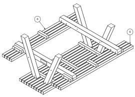
Fit seats using M10x150 coach bolts through seats into main support. Use washer and nut and tighten to 90% to allow for final adjustment.
