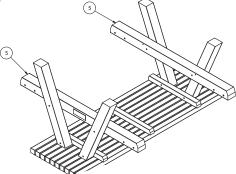
Fit main support members. Face label plate outwards and larger 14mm holes inwards on both. Use M10x170 coach bolt through legs into support member. Use washer and tamper proof nut and tighten to 90% to allow for final adjustment.
