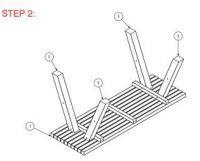
To attach the legs, fit the M10x150 coach bolts supplied through the legs then table top. Tighten washer and nut 90% (to allow for final adjustment)
